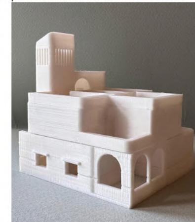
Printing a unit as a whole to mimic on site printing.
